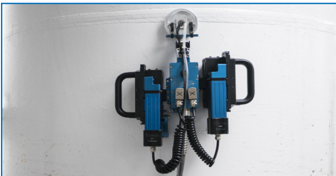
Tank and Vessel Corrosion Inspection Version
